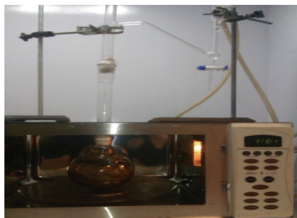
Fig. 1. A microwave-assisted extraction set-up (containing, retort stands, condensers and flat-bottomed flask holding the samples under extraction).
